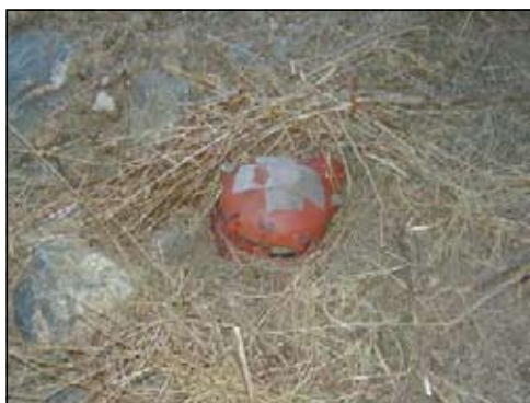
Example of an unprotected wellhead.
