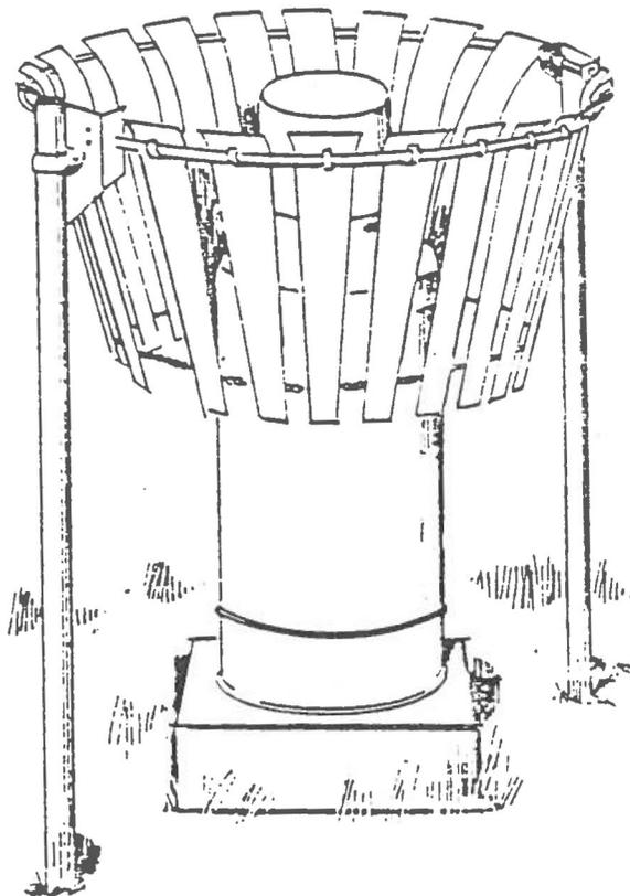
Figure 6 - Shielded rain gauge
