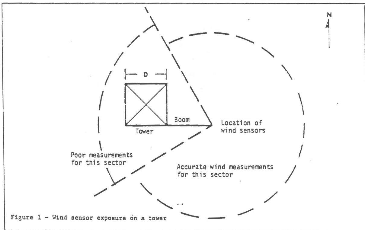
Figure 1 - Wind sensor exposure on a tower
