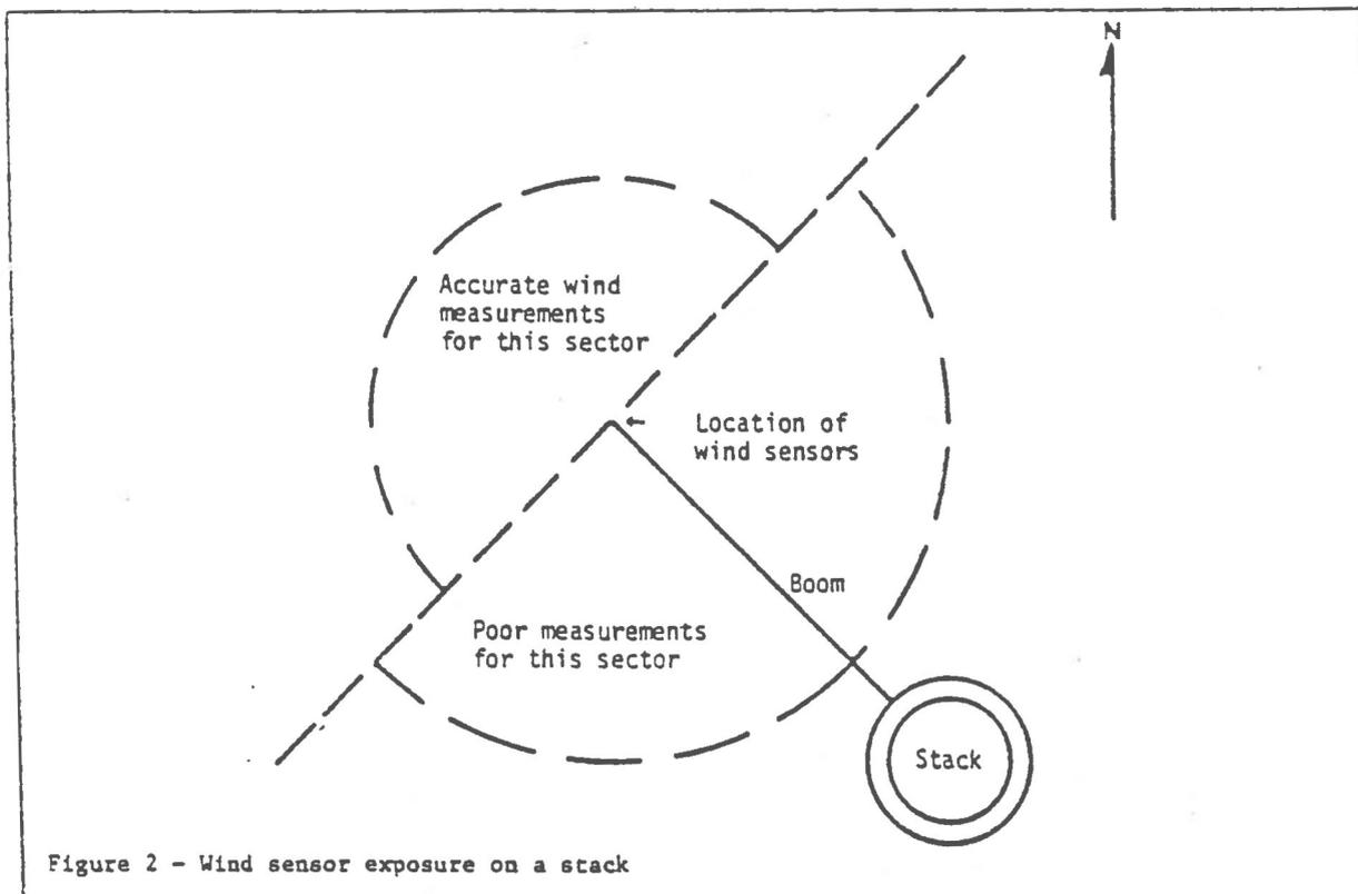
Figure 2 - Wind sensor exposure on a stack
