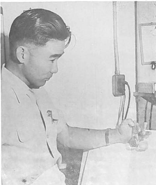
Lower left - Dark vial on left illustrates soil with plentiful supply of available phosphorus. The vials are placed in a colorimeter which accurately measures intensity of color.
