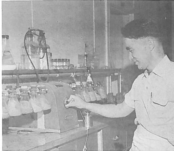
Above - Shaking the soil sample and baking soda solution with a mechanical shaker. The entire test can be completed in less than one hour.
