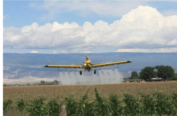
Fig. 2 Treatments were aerially applied using an Air Tractor 402B configured with an ASC rotary atomizer nozzling system. The application was made at 3 gallons/acre.
