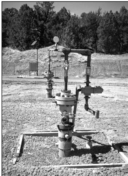
Figure 12. Coalbed methane well surface equipment (i.e., Christmas tree), La Plata County, Colorado. (Photo by Laura Wray)
