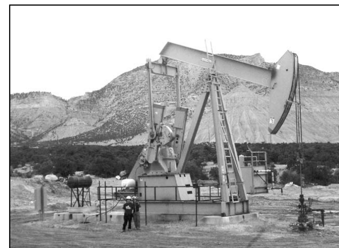
Figure 11. Surface pumping unit (pumpjack) on an Upper Cretaceous coalbed methane well. (Photo by Laura Wray)
