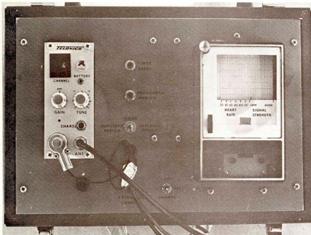
Fig. 2. Receiver and strip-chart recorder used to receive heart-rate signals. (Photo by D. J. Freddy)
