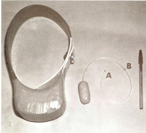
Fig. 1. Transceiver neck-collar, left, and heart-pulse transmitter, right, used to monitor heart-rates of deer. Two stainless steel electrodes exit from transmitter within a protective teflon plastic tube and surface outside the tube (points A and B) to contact animal tissue. (Photo by F. Waugh)
