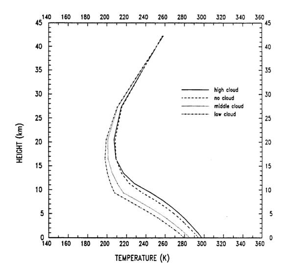
Figure 4.17: Vertical distribution of radiative convective equilibrium temperature for various types of cloud condition.
