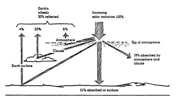
Figure 2.4: On the average, of all the solar energy that reaches the earth's atmosphere, about 30 percent is reflected back to space, 19 percent is absorbed by the atmosphere and clouds, and 51 percent is absorbed at the surface. (after Ahrens, 1981)
