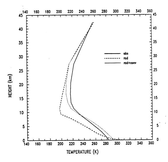
Figure 4.9: Temperature profile of actual atmosphere (solid curve), pure radiative atmosphere model (dash curve), and radiative convective atmosphere model (dot curve).
