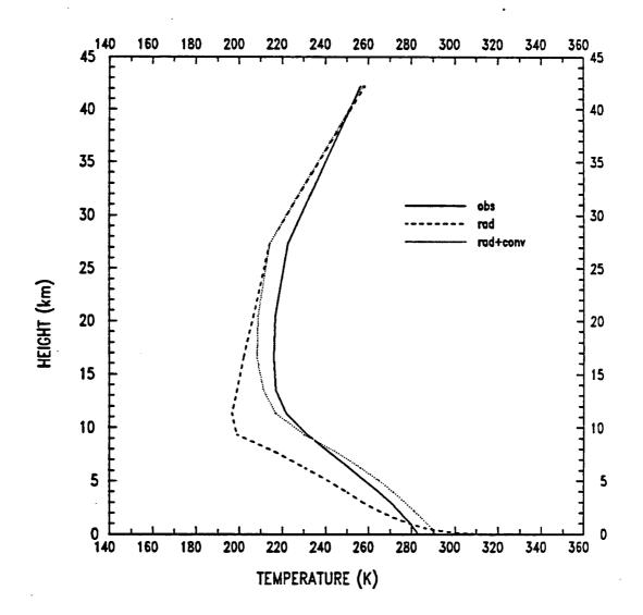
Figure 2.10: Temperature profile of actual atmosphere (solid curve), pure radiation atmosphere model (dash curve), and radiative convection atmosphere model (dot curve).
