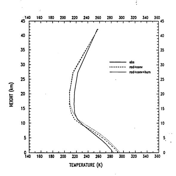
Figure 4.12: Temperature profile from real atmosphere (solid), experiment 2 (dash), and experiment 3 (dot).
