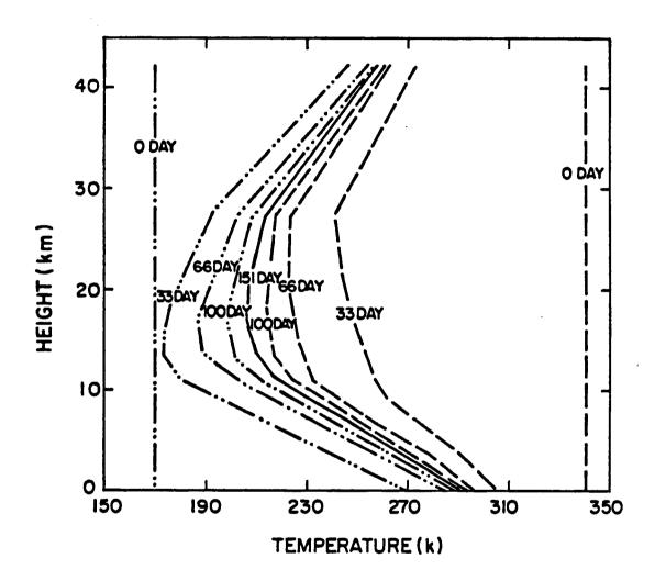
Figure 4.8: Approach to radiative convective temperature profile from two initial isothermal atmosphere at 170k and 340k.
