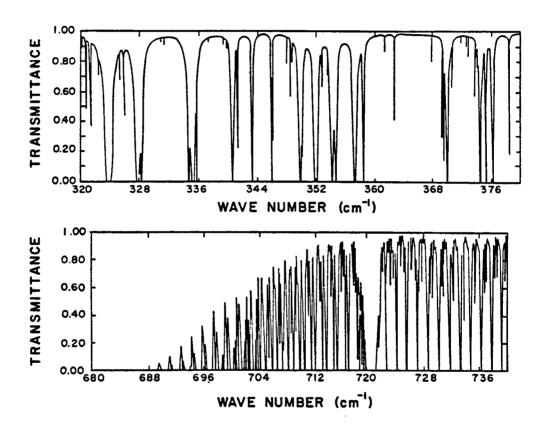
Figure 2.6: Absorption spectrum of the water vapor rotational band and 15  $\mu m$  carbon dioxide band at high resolution (after McClatchey and Selby, 1972).
