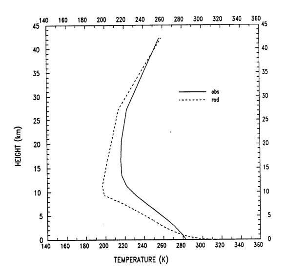
Figure 4.6: Temperature profile of the real atmosphere (solid curve) and pure radiative atmosphere model (dash curve).
