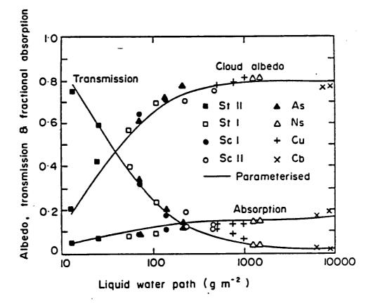
Figure 2.8: Comparisons between the shortwave absorption, transmission and cloud albedo as determined by the theoretical model for the given water cloud types (illustrated points) and the parameterized scheme (solid lines). The cosine of the solar zenith angle  $(\mu_o)$  is 0.8 and a zero surface albedo  $(\alpha_s)$  is assumed (after Stephens, 1978).
