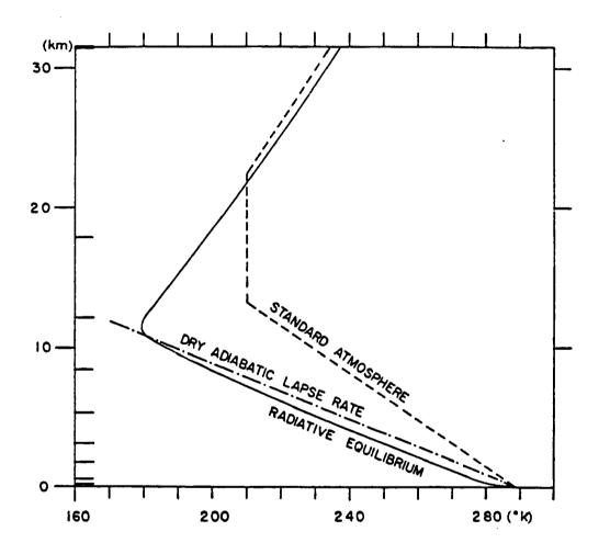
Figure 4.7: Distribution of radiative equilibrium temperature. The amount of sunshine, the distributions of gases, and surface temperature at 30° N in April were used ( $\delta = 0.03^{\circ}C/day$ ). The line of standard atmosphere and that of dry adiabatic lapse rate are also shown for the sake of comparison (after Manabe and Moller, 1961).
