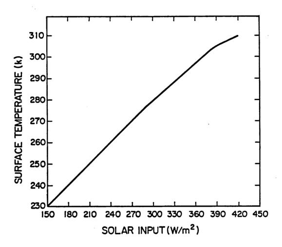
Figure 4.13: Solar input and surface temperature of radiative convective equilibrium.
