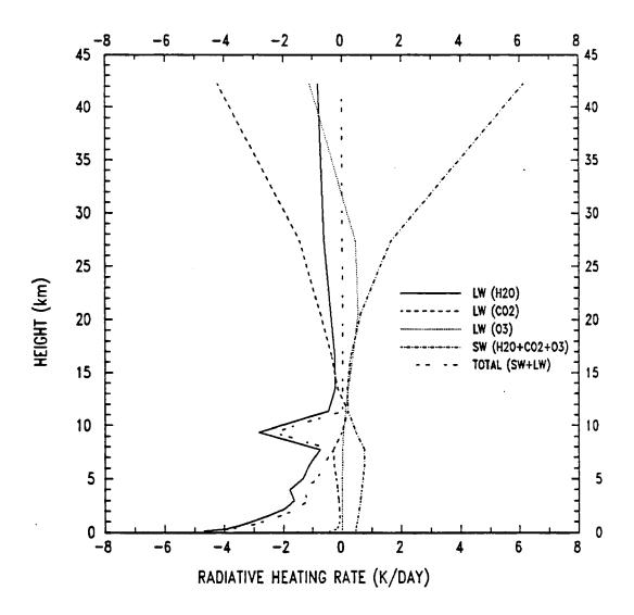
Figure 4.11: Vertical profiles of various equilibrium radiative heating rate.
