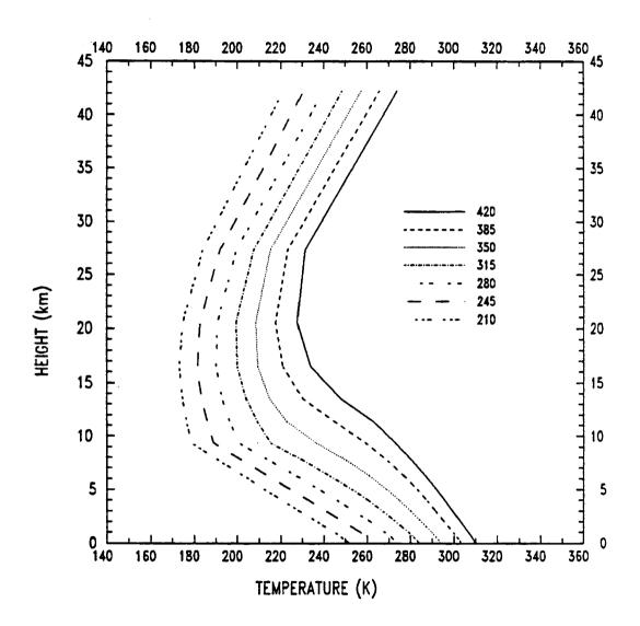
Figure 4.14: Vertical distribution of radiative convective equilibrium temperature of the atmosphere for various values of solar input.
