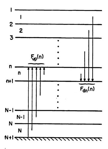
Figure 2.5: Illustration of infrared upward and downward fluxes at level Z.
