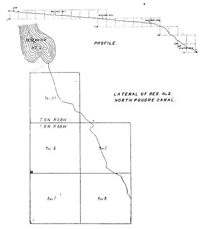
For the first mile the canal had a fall of 5.4 feet, in the econd mile 4.8 feet, in the third mile 5.8 feet and in the last nile 34 feet. The reason for this rapid increase of grade 5, that for the first three miles the ditch skirts the side of a divide, while a short distance after passing the third nile post it reaches the ridge of the divide and descends with the slope of the country which is quite abrupt.
