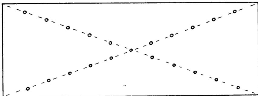
Showing a good plan for distributing samples over a field
