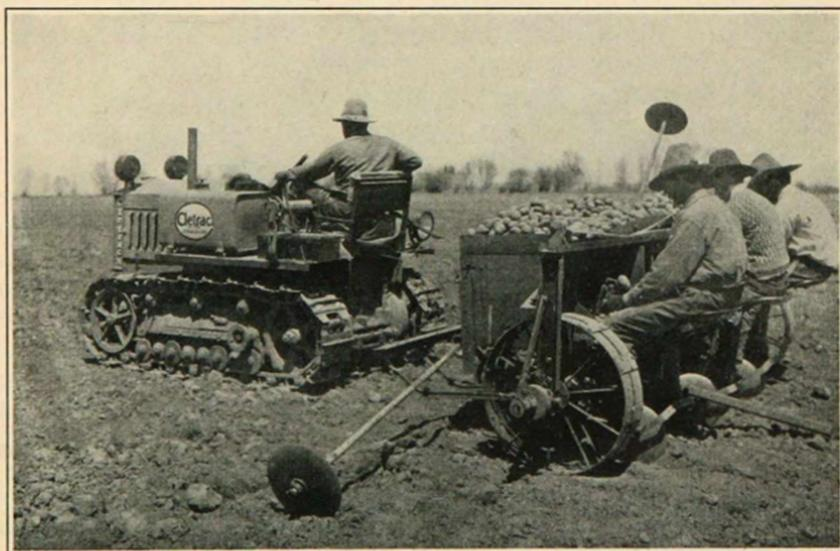
Figure 52. Three-row cup-type potato planter and men to correct the feed.
