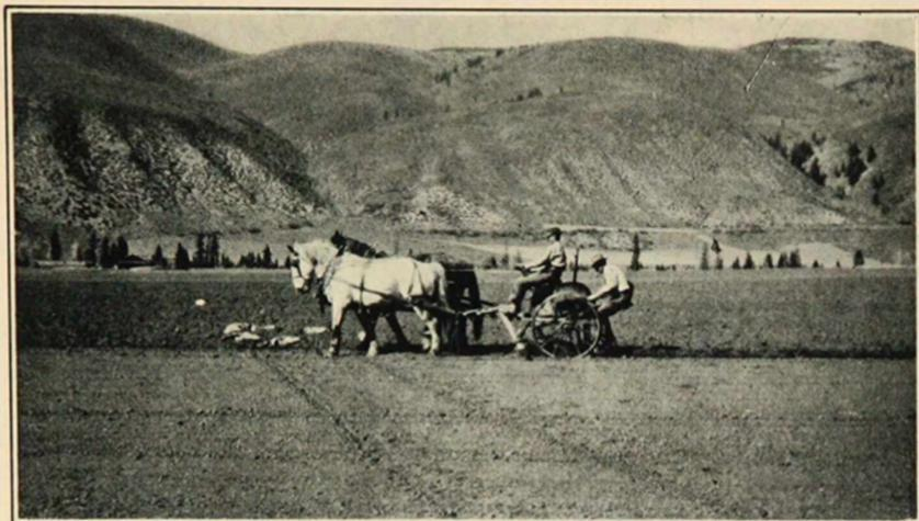
Figure 54. Two-man or assisted-feed potato planter.
