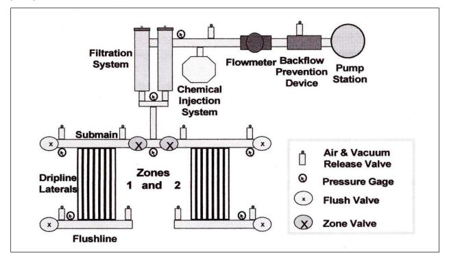
Figure 8. Typical drip irrigation system configuration (http://www.oznet.ksu.edu/sdi/)
