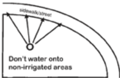
Figure 3. Avoid placing sprinkler heads in the center of the lawn.
