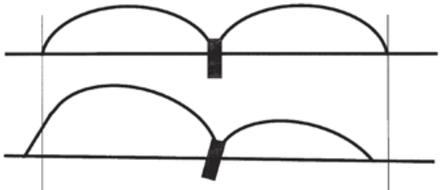
Figure 7. Make sure to monitor sprinkler performance often as the water distribution can change when the head tilts.
