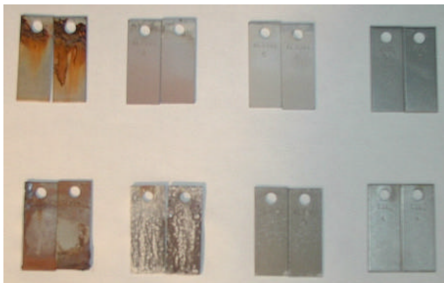
Fig. 2-16 Coupons after the NACE test
