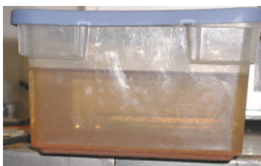
Fig. 2-13a The 3 wt.% \text{MgCl}_2 solution used in the SAE test after 20 days
