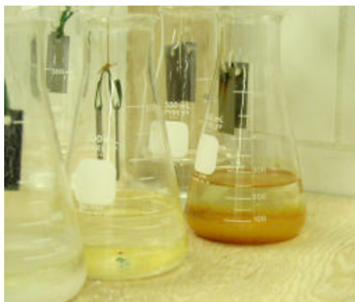
Fig.2-11b The MgCl_2 solution in the NACE test ( at 69 days)
