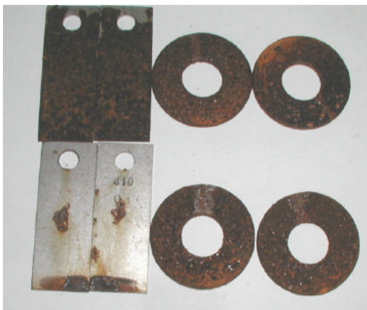
Fig. 2-24a Coupons by the SAE test without the dry stage after 7 days (upper: by \text{MgCl}_2 ; lower: by \text{NaCl} )
