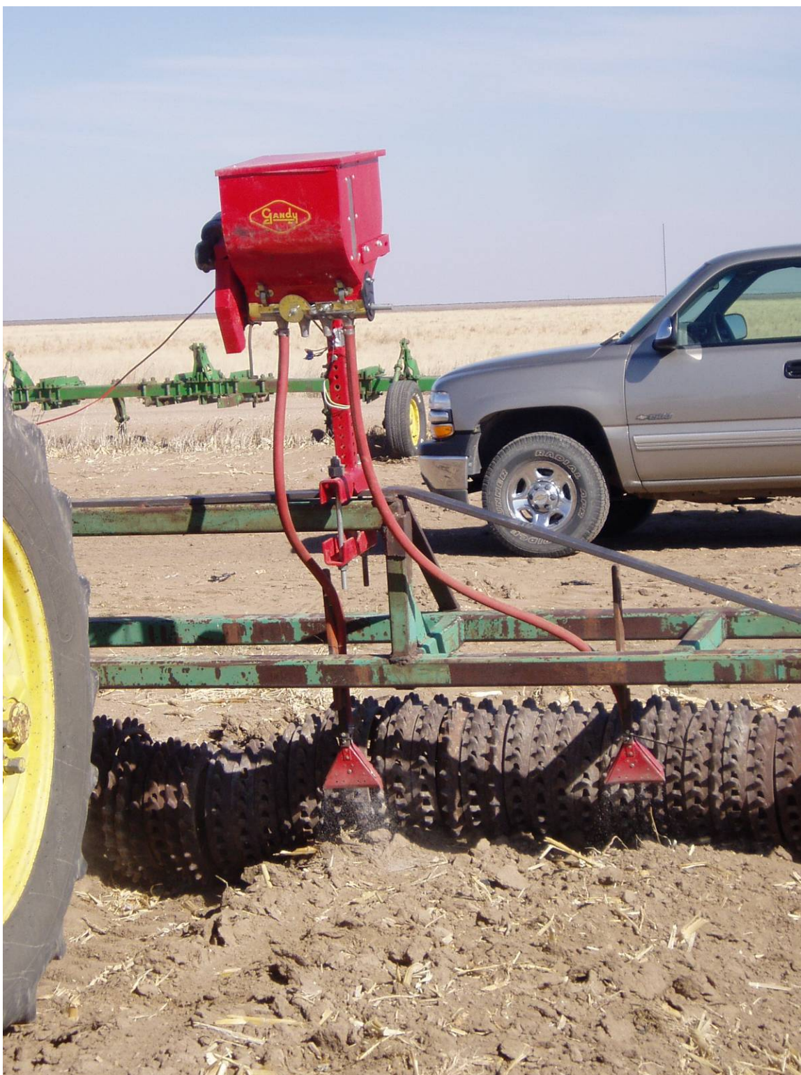
Picture 5. Gandy Box feeding AgriBlend above driplines.
