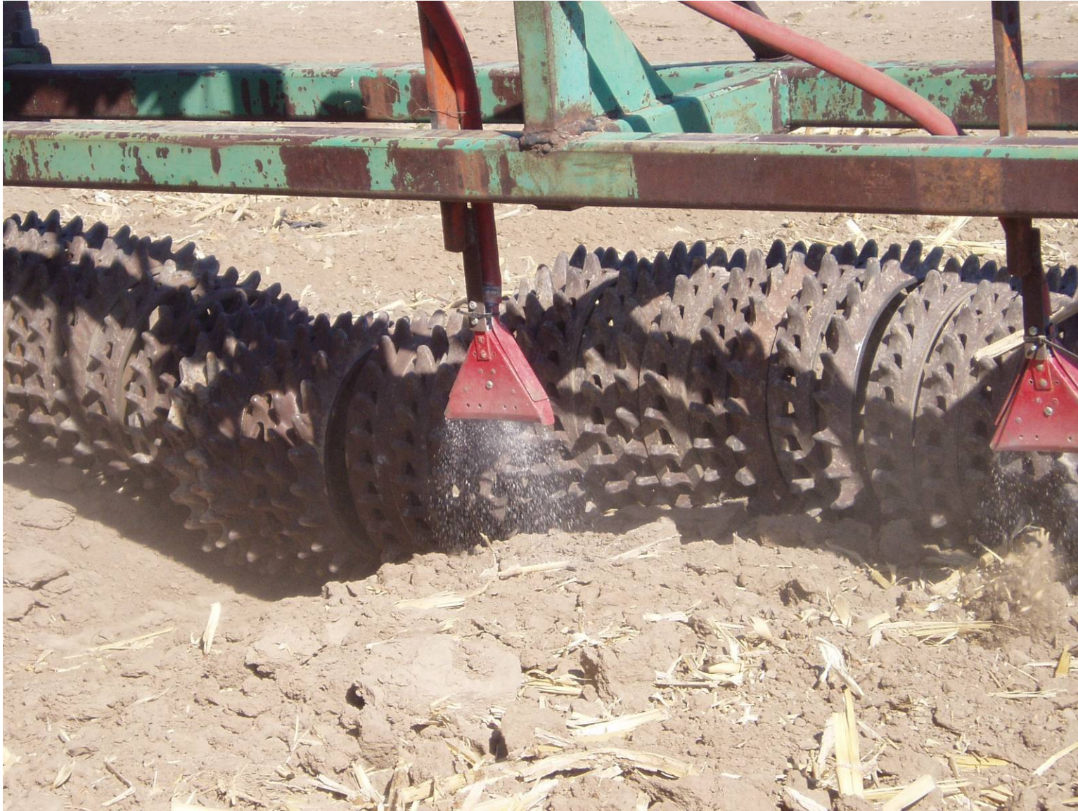
Picture 6. AgriBlend being fed through fan applicators.
