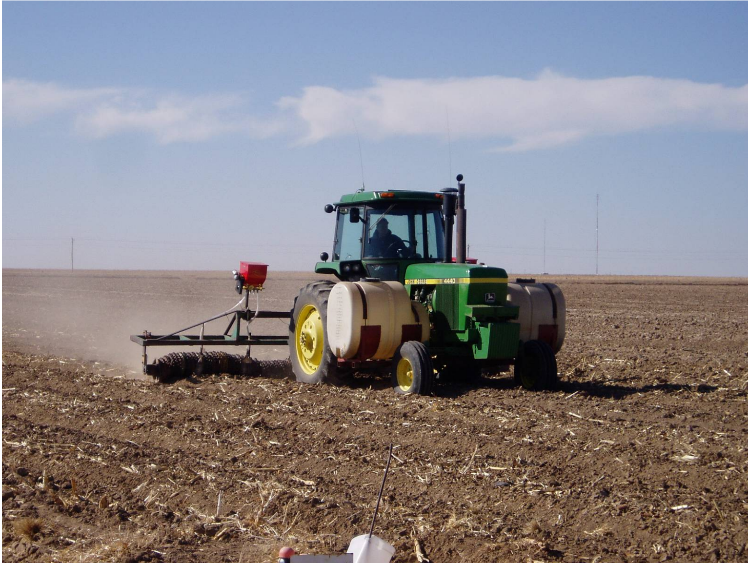
Picture 7. Culti-packer used to work beds and incorporated AgriBlend.
