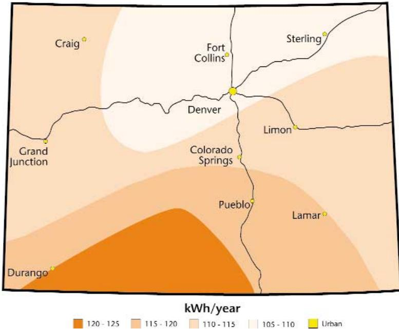
This map shows the thermal output of a solar hot water system in metric units based on a per-unit rating of the capacity of the solar panels (per thousand British thermal units per day [kBtu/d]). You can compare this output with that of a conventional electric water heater.
