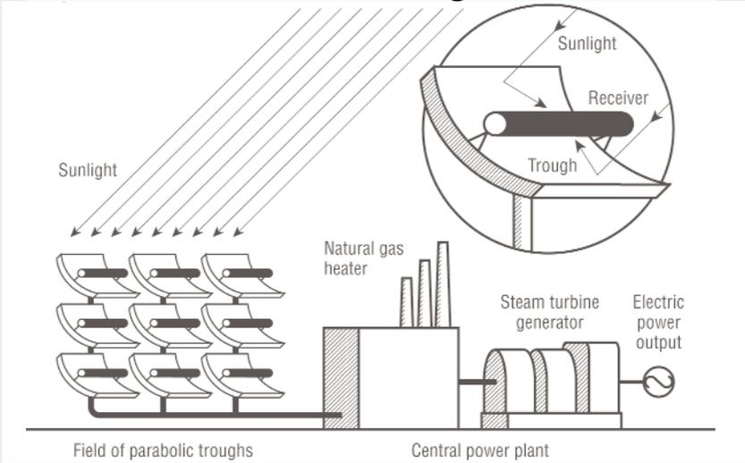
Parabolic troughs collect the sun's energy as heat for generating electricity in a conventional steam turbine.
